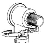
Attach the levers (H) to the locking pins positioned at the rear of the same, ensuring that the upper cavity fits onto the link (F).
