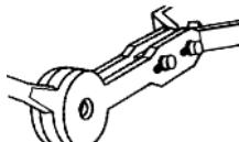
Join the locking key (A) between the two levers (H) provisionally leaving the pins in the large slots.
