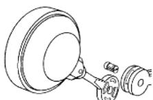
Attach the levers (H) and the float (L) pushing the pin (I) into the special slot applying pressure until it clicks into place.
