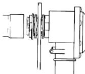
Assemble the elements as shown in the diagram and tighten the threaded washer (D) without forcing it.
