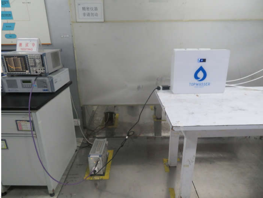
TERMINAL DISTURBANCE VOLTAGES TEST SETUP
