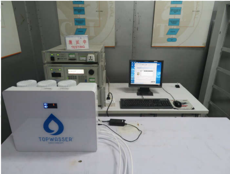
VOLTAGE DIPS AND INTERRUPTIONS TEST SETUP
