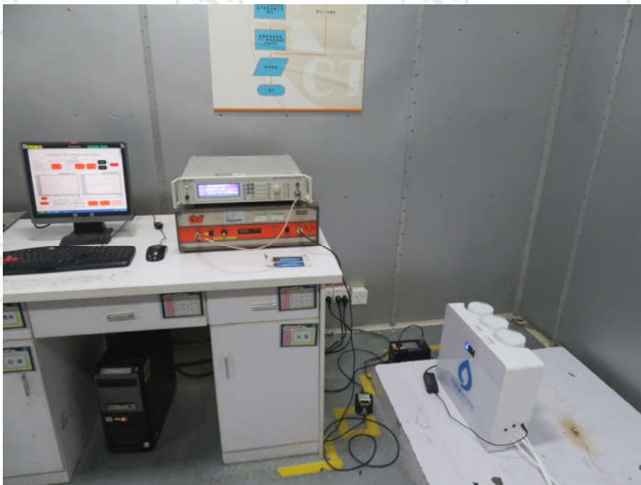
INJECTED CURRENTS TEST SETUP
