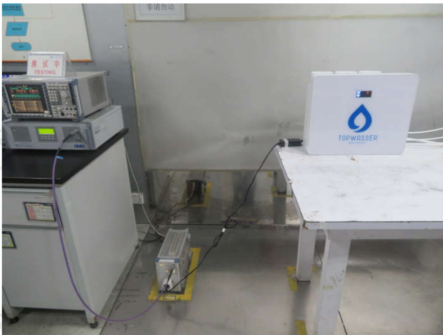
DISCONTINUOUS DISTURBANCE (CLICKS) TEST SETUP
