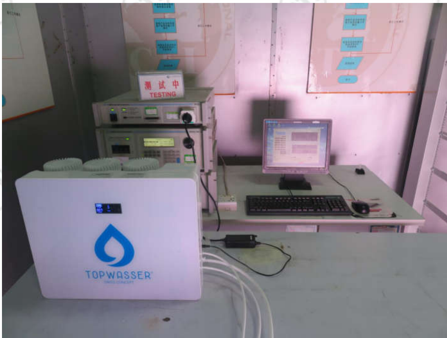
HARMONIC & FLICKER TEST SETUP
